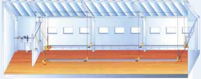
A slope neutralizer can be mounted in the middle of the line to correct any pressure modification due to the farm floor inclination
